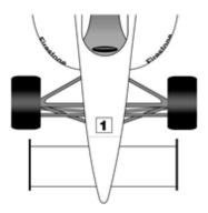
4.5.3.9. Headrest - The Car number must be a minimum dimension of 1 inch by 1 inch. The Car number must be located on top of the headrest behind the Driver's helmet in a contrasting color (See Illustration).
