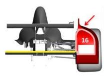
**4.5.3.11.2.** The minimum height of the numeric digit must be 8 inches and the width of the numeric digit must be a minimum of 1 inch of continuous color. The numeric digit must be no less than 9 inches from the top (**See Illustration**).
