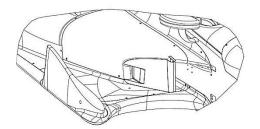
b) Dallara Blanking Panel –This part may be manufactured by an Entrant or purchased from Dallara. Panels must be mounted perpendicular to the car centerline in the approved location at the entrance to the radiator inlet duct.
