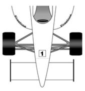
**4.5.3.6. Headrest** - The Car number must be a minimum dimension of 1 inch by 1 inch. The Car number must be located on top of the headrest behind the Driver's helmet. Letters and numbers must be in Impact font, black or white in color, and no trim is permitted. **(See Illustration).**
