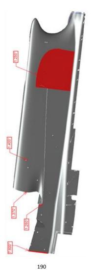
**14.6.6.8.** For all others Events, the underwing step plane heights must adhere to the following illustration. The heights of 1.200 inches, 1.250 inches, 1.370 inches, and 1.400 inches have a tolerance of plus 0.200 inches and minus 0.00 inches.
